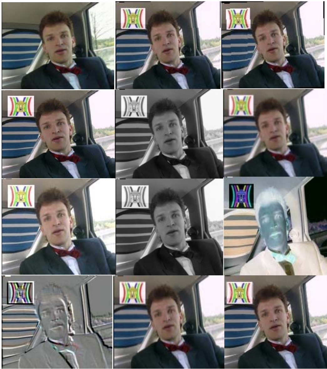
Fig. 6. The example of attacked video Vid2 . From top-line to bottom-line: No attack, Rotation w. crop ( 1^0 ), Rotation w. crop ( 2^0 ), Scaling 1.0-2.0-1.0, Grayscale, Blur, Brightness & Contrast, TV Y-channel, Invert Color, Smoother, Emboss, Deinterlace
