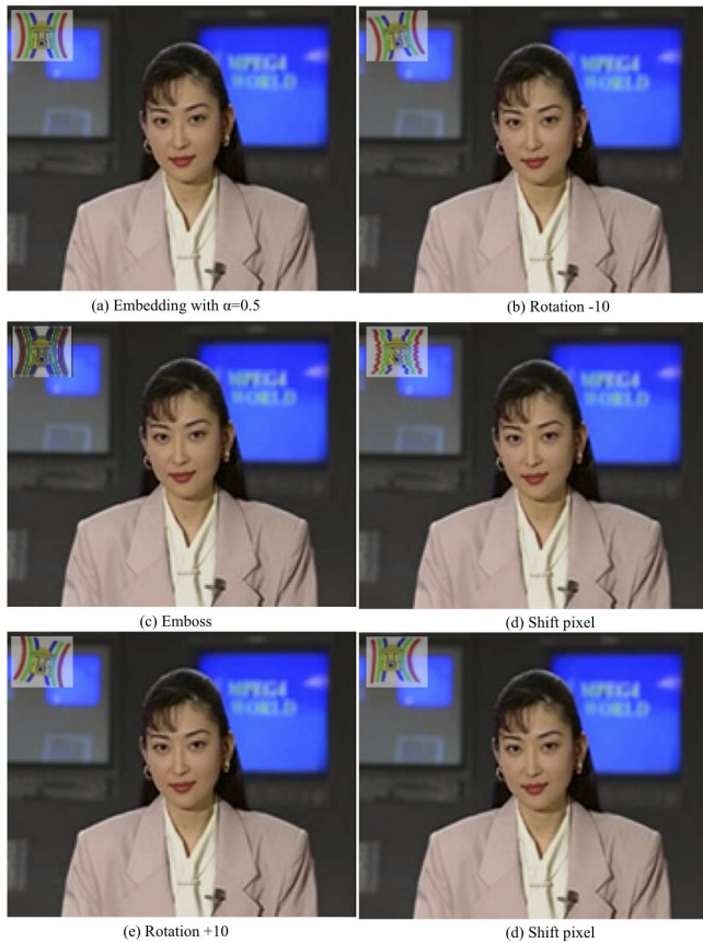
Fig. 3. The embedding of visible watermarking. The distorted logos are created by GIMP 2.8. If shot change is detected, the visible logo is randomly embedded. The embedding strength \alpha = 0.5 .
