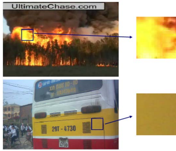
Fig. 4. Spatial variation in fire and in a fire-like coloured object
