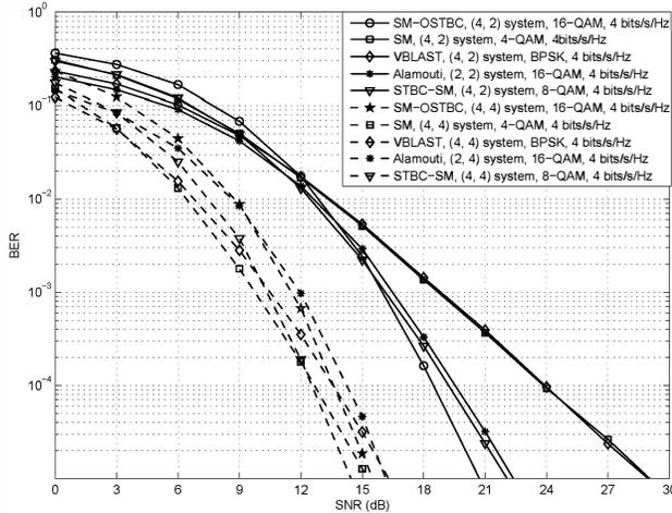
Fig. 3. BER curves of the proposed SM-OSTBC in comparison with those of SM, VBLAST, the Alamouti's STBC, and STBC-SM; 4 bits/s/Hz.
