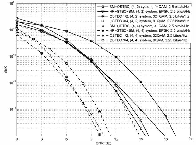
Fig. 2. BER curves of the proposed SM-OSTBC, HR-STBC-SM, and OSTBC 1/2 at 2.5 bits/s/Hz and OSTBC 3/4 at 2.25 bits/s/Hz in (4, 2) and (4, 4) systems.
