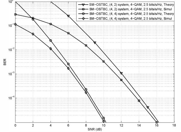
Fig. 1. Theoretical upper bounds and simulation results of BER performance of the proposed SM-OSTBC scheme for different numbers of receive antennas.
