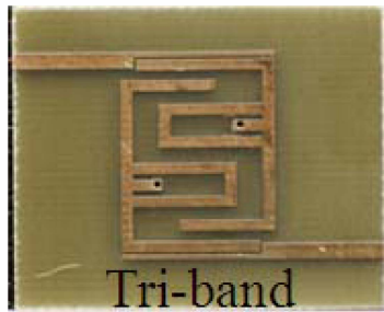
Fig. 5 Photograph of the fabricated tri-band bandpass filter.
