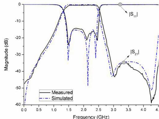
Fig. 5. Measured and simulated results S parameter of the wideband bandpass filter.
