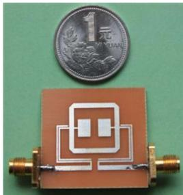
Fig. 7 Photograph of the fabricated wideband BPF.
