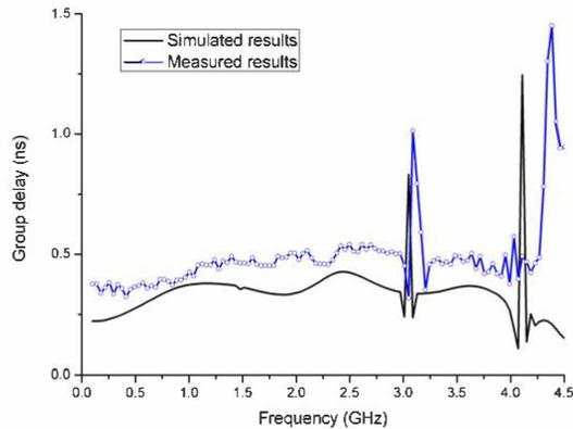
Fig. 6. Measured and simulated results group delay of the wideband bandpass filter.
