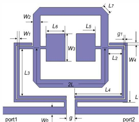
Fig. 1. Layout of the proposed wideband bandpass filter.
