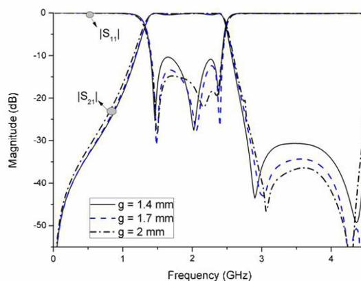
Fig. 4. Simulated frequency response  $|S_{11}|$  and  $|S_{21}|$  of the filter under different values of  $g$
