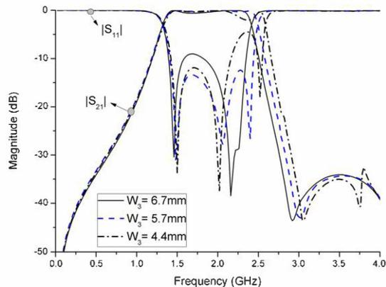
Fig. 3. Simulated frequency response  $|S_{11}|$  and  $|S_{21}|$  of the filter under different values of  $W_3$
