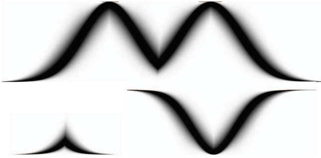
Fig. 6. Outputs of operations of G-T2FS; the top: JOIN; the left-bottom: MEET and the right-bottom: NEGATION
