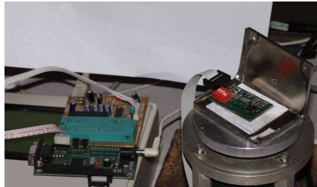
Figure 3. 3-DOF Piezoresistive accelerometer testing on the shaker, vibrated signal is then transmitted to \mu -controller.
