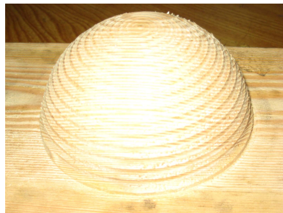
Figure 6. Real cut path on 5-axis CNC machine
