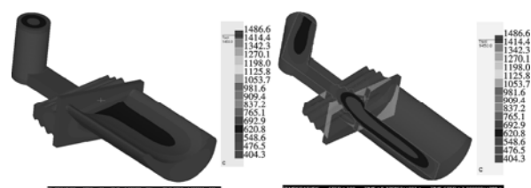
Fig.5 Temperature distribution when corresponding time is 52.70 s
