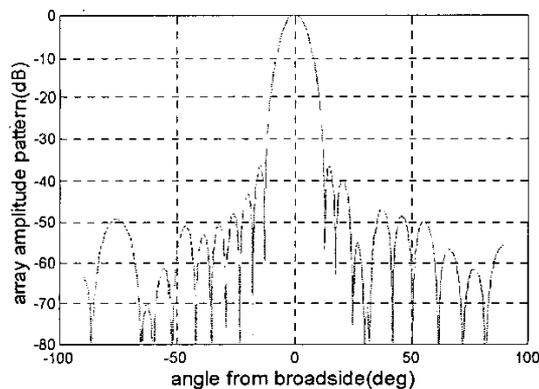
Fig. 3. The synthesized pattern the localized nulls at  $-65^\circ$ ,  $-60^\circ$ ,  $25^\circ$   $30^\circ$
