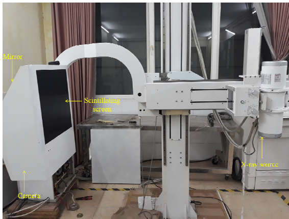
Fig. 2. Our prototype DR with an indirect DSLR-based detector.
