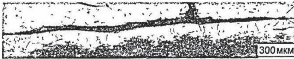
FIGURE 5. Optical image of a fatigue crack in 2CR31 + NI-CR-B-SI composition in the “base-coating” interface region
