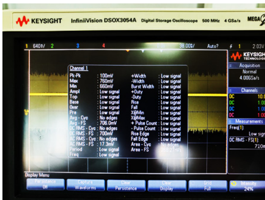
Fig. 22. Detailed information of the measured output voltage waveform shown in Fig. 21.
