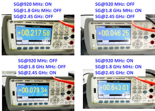
Fig. 20. Measured output DC voltage according to different states of RF signal generators.
