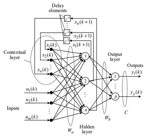
Fig. 1. Architecture of Elman neural network
