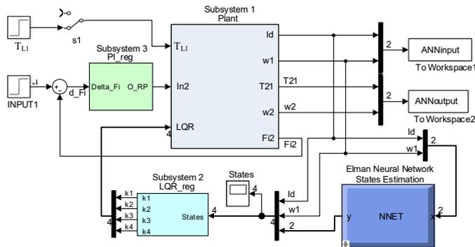
Fig. 3. A simulation model of a closed system in the MATLAB / Simulink
