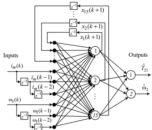
Fig. 2. The architecture of Elman's neural network observer
