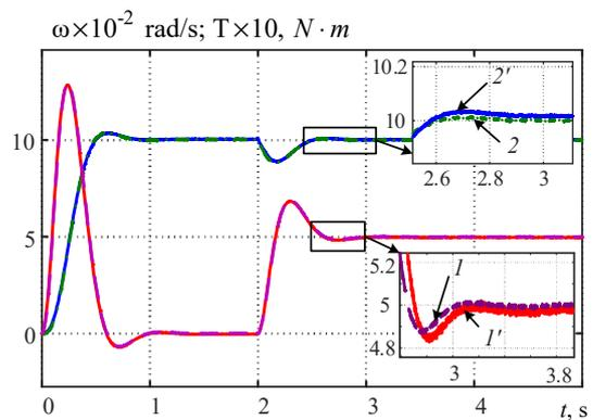
Fig. 6. Estimation results with the Levenberg - Marquardt training algorithm (*trainlm*)
