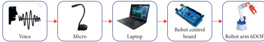
FIGURE 1: Diagram of voice control for the 6DOF manipulator arm.
