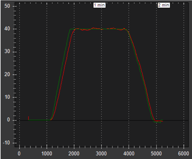
Fig. 10. The difference between desired and actual altitude of drone, green line – desired altitude, red line – actual altitude
