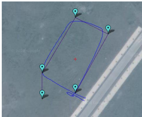
Fig. 6. The difference between desired and real trajectories (pink line – desired trajectory, blue line - real trajectory)
