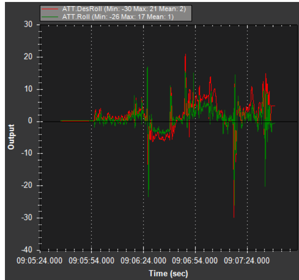
Fig. 7. The pilot's desired roll angle in degrees – red line, the drone's actual roll in degrees – green line
