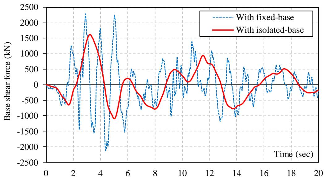
**Figure 12.** Dynamic base shear force in Y direction.
