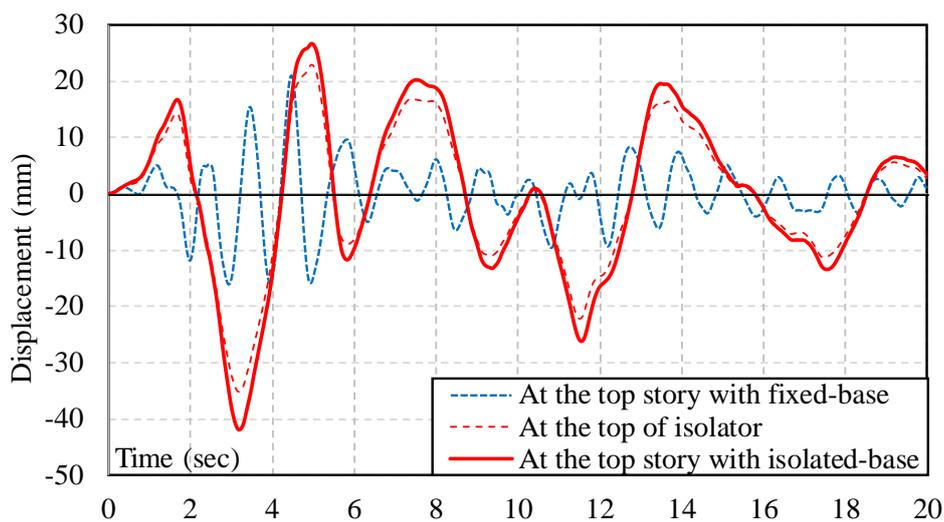
**Figure 14.** Dynamic absolute displacement at the top story (column 1B) in Y direction.
