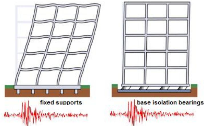
**Figure 2.** Effects of SBI on contour deformation of the structure.
