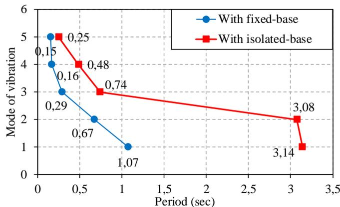
Figure 9. Model periods of structures' vibration.
