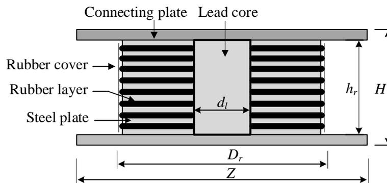
**Figure 3.** Structure of lead-rubber bearing isolator.
