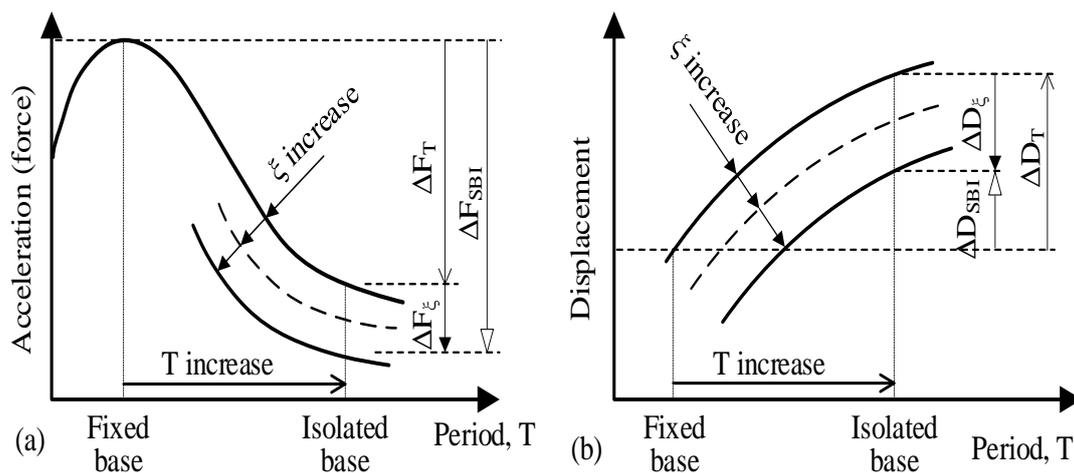
**Figure 1.** Effects of SBI approach on the seismic responses: (a) on spectral acceleration (lateral force), (b) on lateral displacement.
