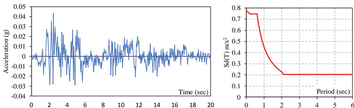
**Figure 8.** Spectrally acceleration time history and horizontal design spectrum used for study.
