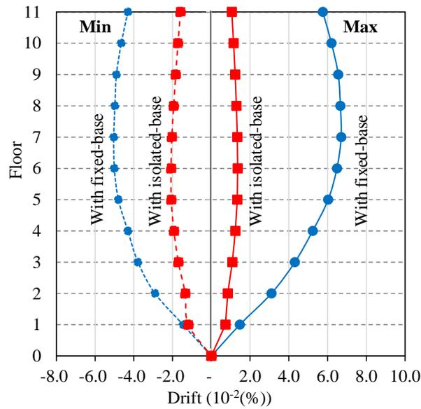
**Figure 11.** Story drift diagram of building subjected to seismic action in Y direction.
