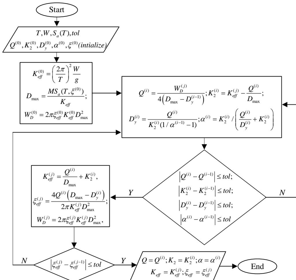
Figure 6. Iterative design procedure for determination of SBI properties.
