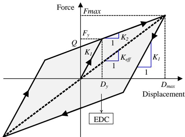
Figure 5. Parameters of bilinear model.
