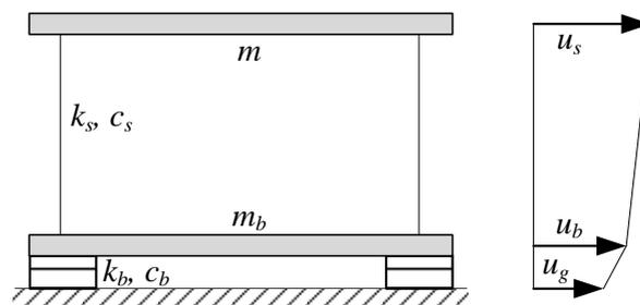
**Figure 4.** Simplified structural model of two-degrees-of-freedom isolated system.
