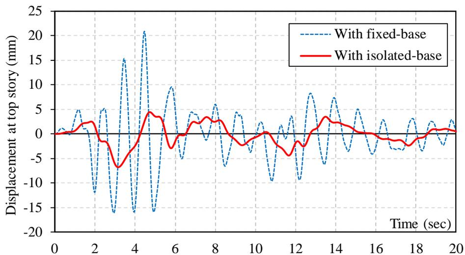
Figure 15. Dynamic relative displacement at the top story (column 1B) in Y direction.
