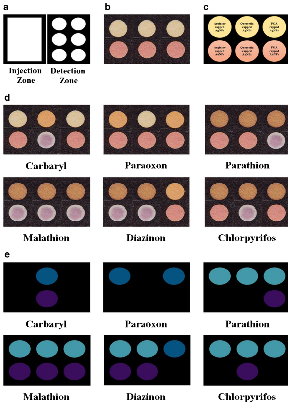
Fig. 1 a The schematic of designing PAD. b The image of the fabricated sensor array. c A pattern for the introduction of sensing elements. d Response of sensor and e color profiles for 6 different types of pesticides ( 1.0 \mu\text{g mL}^{-1} ). The experiment was done at optimized conditions (Tris buffer ( 0.5 \mu\text{L} , 0.10 \text{ M} , \text{pH} = 9.0 ) and 0.35 \mu\text{L} of NPs). The response of the sensor was captured after 15-s incubation
