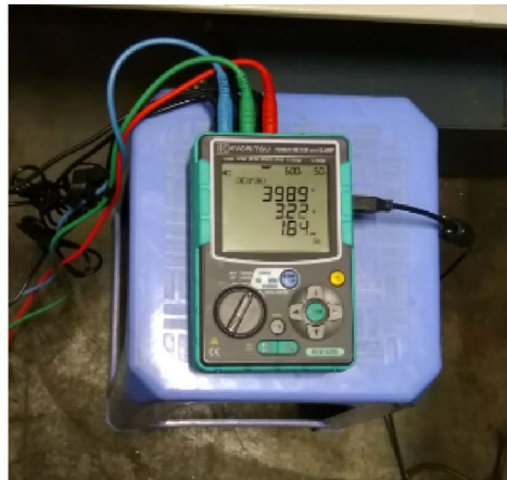
(a) The value of the power consumed by the machine tool at the experimental No. 20 (Replication-2)
