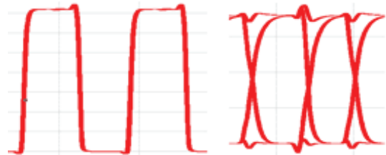
Fig. 10. Jitter performance of recovered clock and data at 3 Gb/s.
