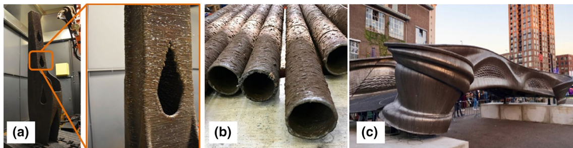
Fig. 1 Some examples of steel thin-walled components and steel components composed of thin-walled features fabricated by WAAM: a the excavator arm [27], b tubular components [28], and c the footbridge [29]
