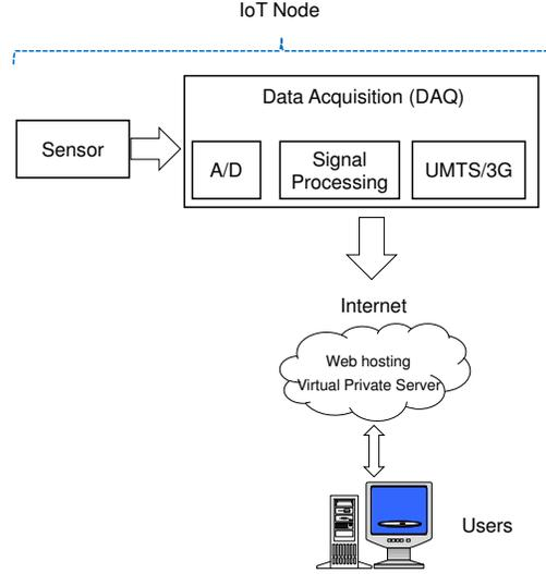
Fig. 4. Structural health monitoring system with IoT nodes.
