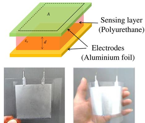
Fig. 1. Structure (the above) and photos of the capacitive pressure sensor in the normal mode (the below left) and flexible mode (the below right).
