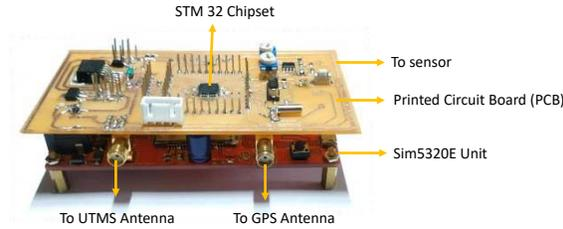
Fig. 6. Picture of the DAQ module with dimensions  $(6 \times 10 \times 4) \text{ cm}^3$ .
