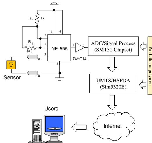
Fig. 5. DAQ's circuit diagram of the SHM system.
