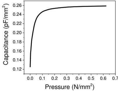
Fig. 2. The capacitance-pressure characteristic of the sensor.
