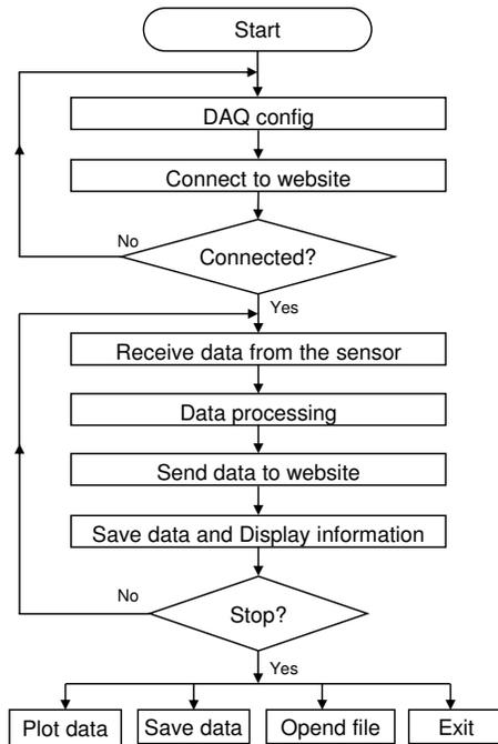
Fig. 7. The operation flow of the proposed system with the integrated software.
