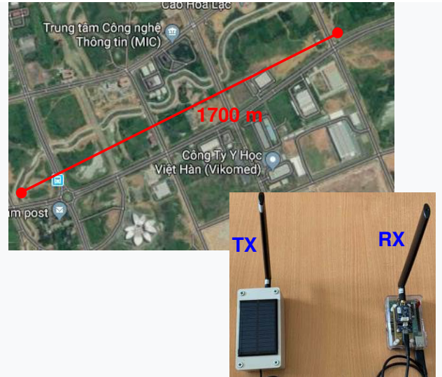
Fig. 4. The demonstrated monitoring system using proposed temperature Beat sensor and LoRa communication protocol.
