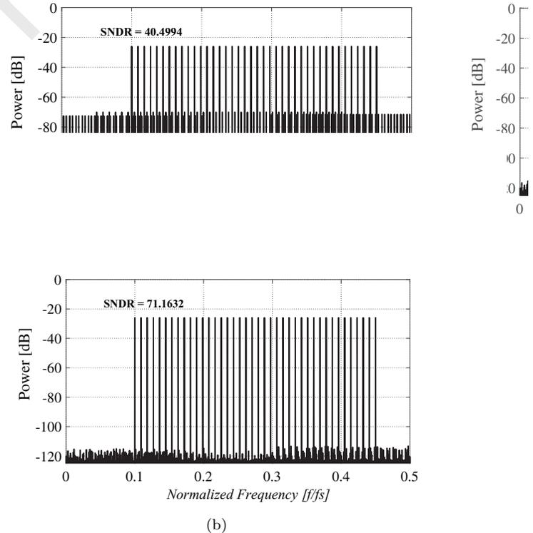
Fig. 7: Output spectra for the band-limited bandpass multitone input: (a) Before calibration; (b) After calibration.
