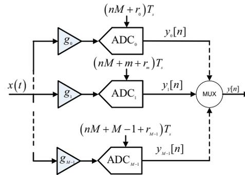
Fig. 1: An  $M$ -channel TIADC with gain and timing mismatches.
