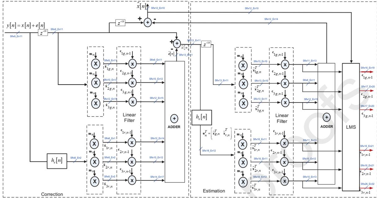
Fig. 14: The optimal fixed-point hardware architecture of the proposed calibration.
