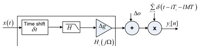
TIADC equivalent to an ADC clocked at a sampling rate of  $f_s = \frac{1}{T_s}$ .
