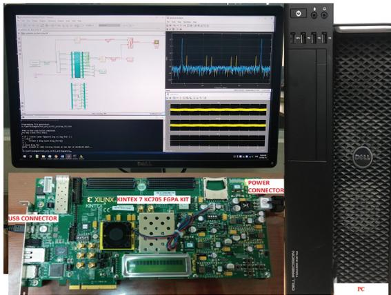
Fig. 15: Experimental platform for FPGA implementation.
