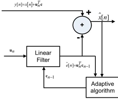
Fig. 2: Digital estimation based on Adaptive Noise Canceller (ANC).
