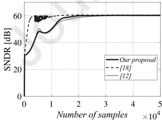
Fig. 11: Time evolution of SNDR during calibration.
