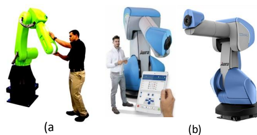
Figure 3: Commercially available collaborative robots of heavy payloads. (a) The cobot CR-35iA made by FANUC Robotics, with the maximum payload of 35 kg [11], and (b) the cobot AURA made by Comau with the maximum payload of 170 kg [12].
