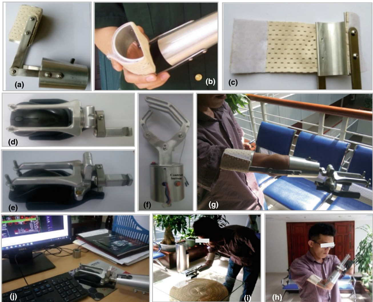
Fig. 5 a–f Successfully developed prototypes of a body-powered prosthetic hand. g–k Evaluation and testing of using a prosthetic hand for the common daily activities
