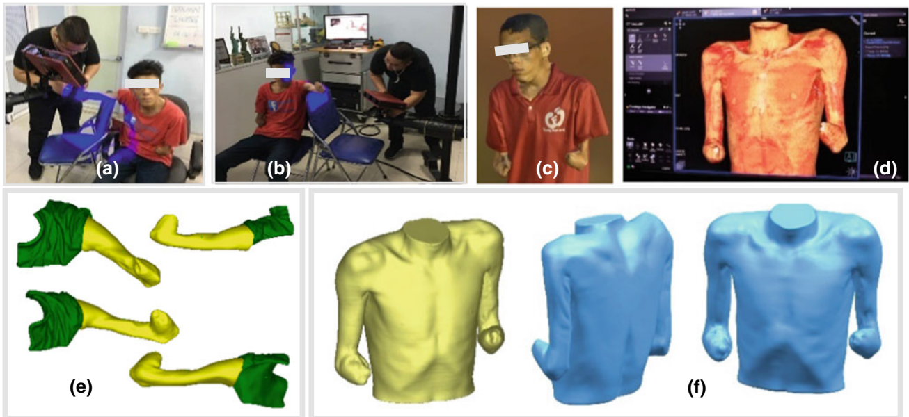
Fig. 2 Data collection and 3D modeling of the body parts for design activities. a, b RE scanning. c, e 3D models constructed from scanned point data. d, f 3D models constructed from CT images
