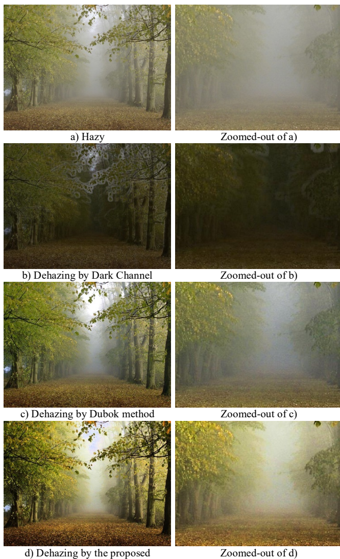
Fig. 4. Dehazing results by the methods for the forest image. NIQE score of the methods: Dark Channel is 2.4261, Dubok is 2.7425, and the proposed is 2.3556 .
