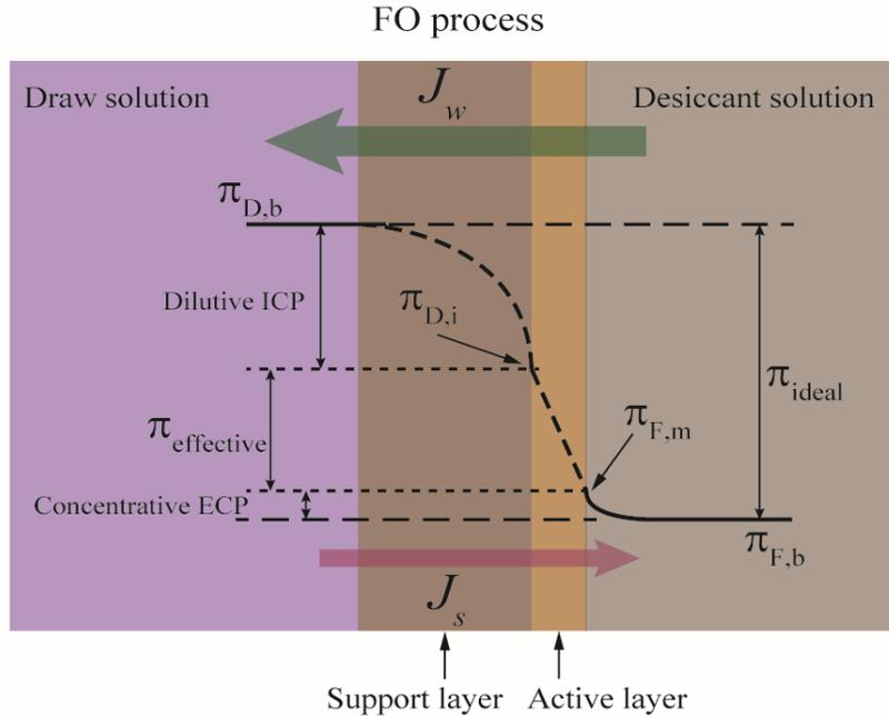
**Fig. 4.** Internal and external concentration polarisation of the FO process.
