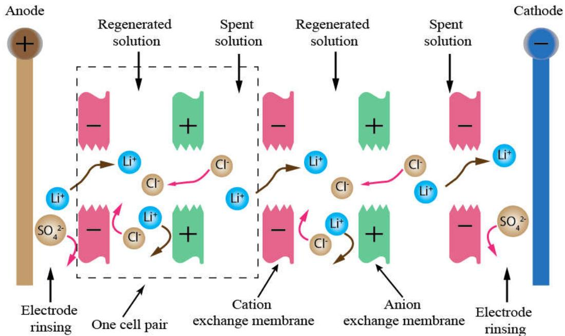
**Fig. 5.** A schematic diagram of an ED process for regeneration of LiCl liquid desiccant solution (adapted from [54]).
