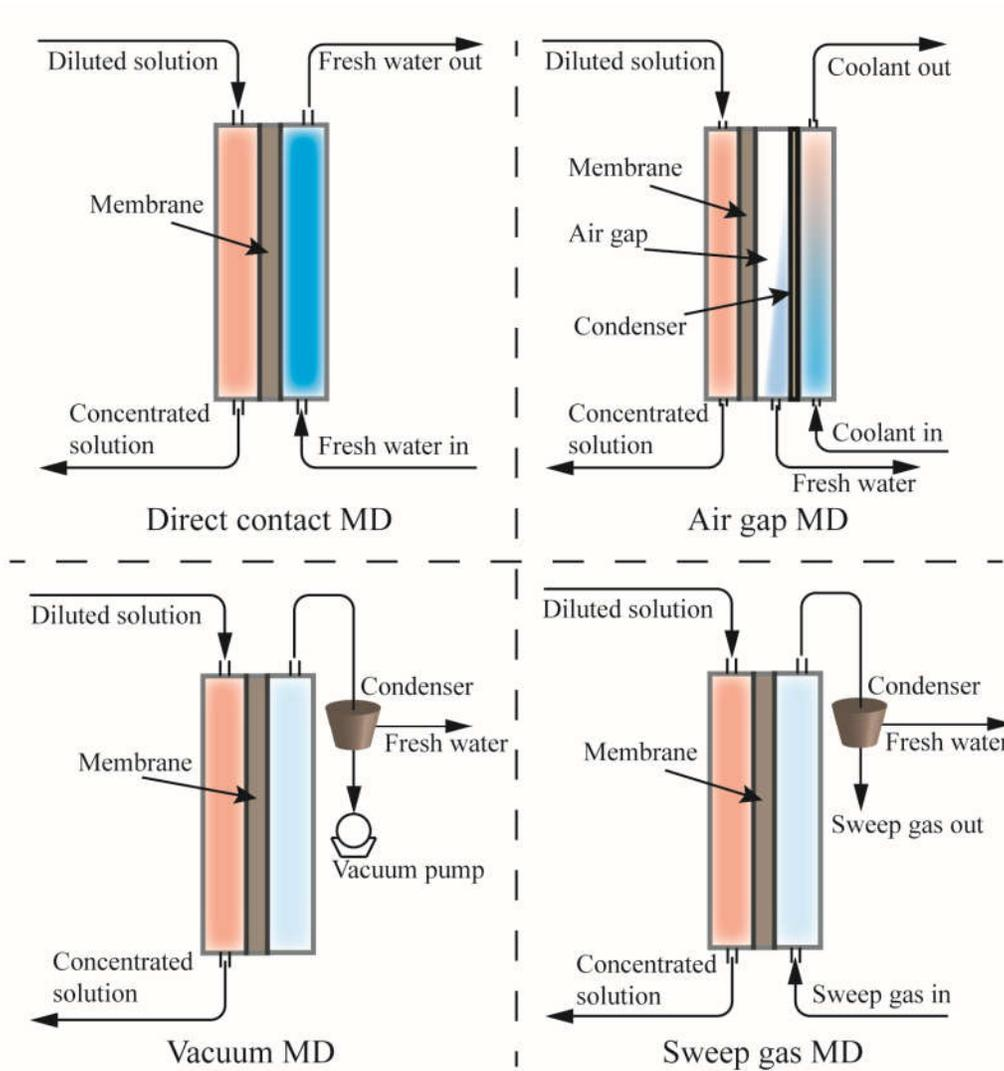
**Fig. 6.** Schematic diagrams of the four basic MD configurations.
