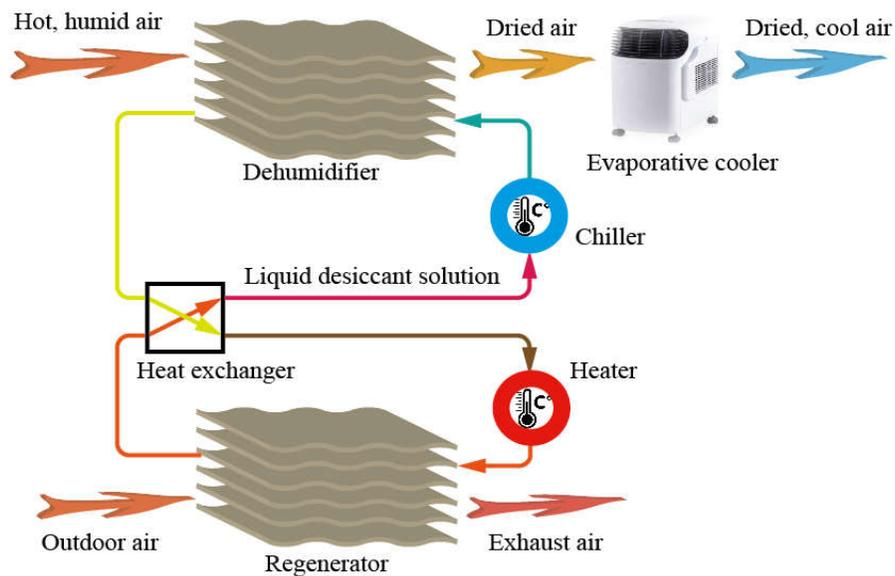
**Fig. 1.** The schematic diagram of a LDAC process.
