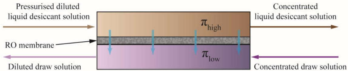
**Fig. 3.** The working principles of the OARO process for regeneration of liquid desiccant solution.
