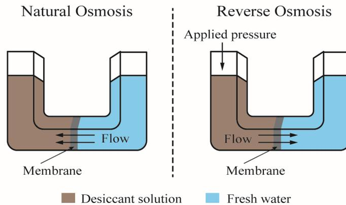
**Fig. 2.** Principles of reverse osmosis for the regeneration of liquid desiccant solution.
