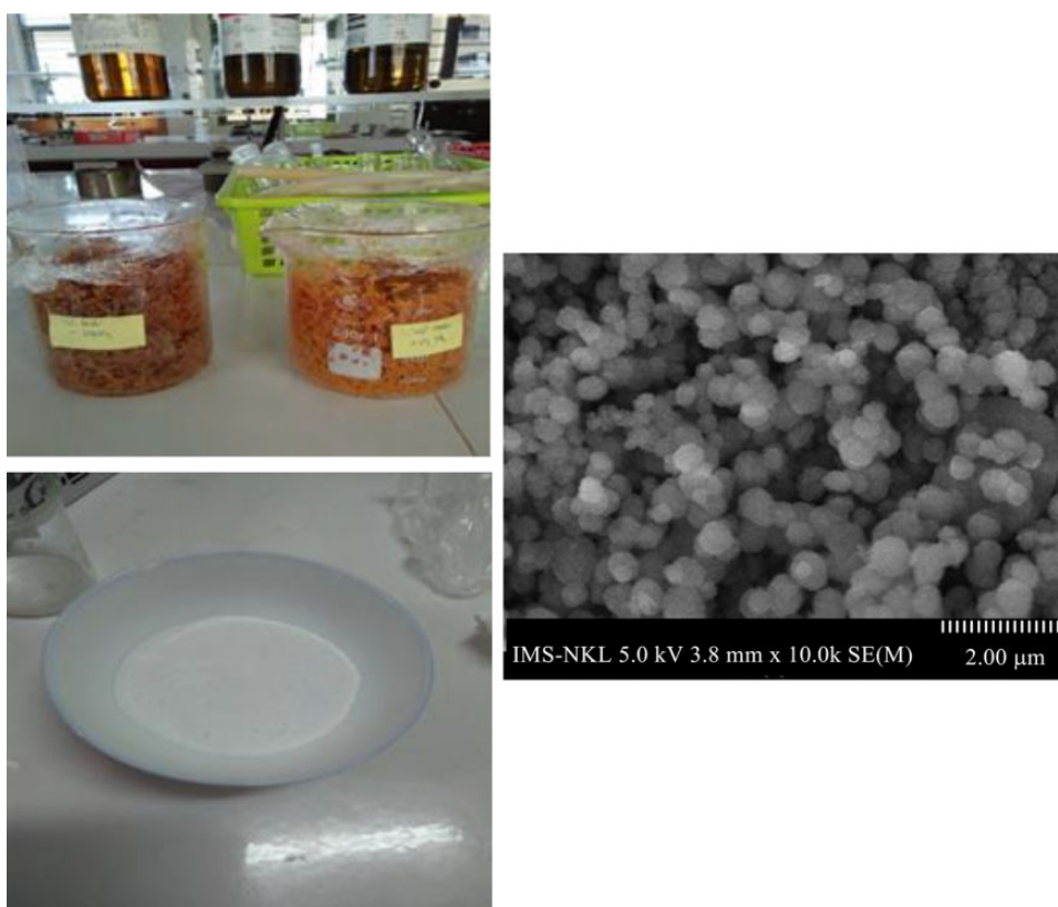
Figure 5. Rice husk in acidic solution, silica rice husk, and scanning electron microscopic image of silica nanoparticles.
