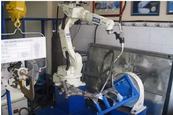
Fig. 1. The welding robot – positioner system FDV8
