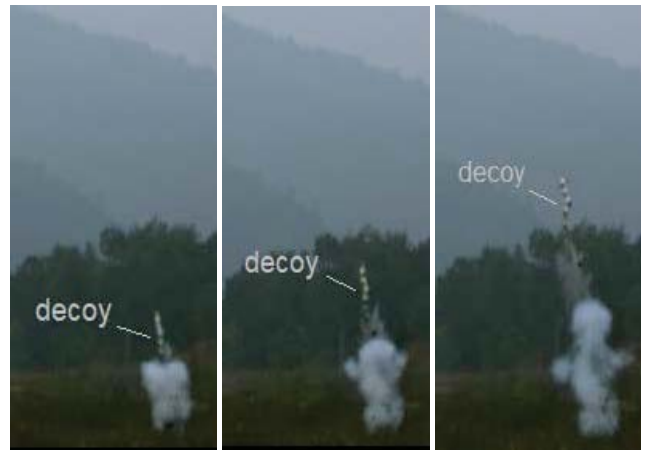
Figure 5. Video imagery of firing test on the prototype of the decoy launcher.
