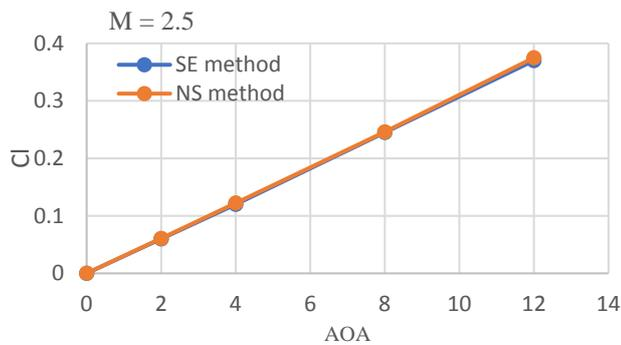
Figure 15. The comparison of lift coefficient results which are determined by two methods Shock-Expansion method and Navier-Stokes method
