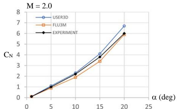
Figure 13. Variation of normal force coefficient with angle of attack [6]
