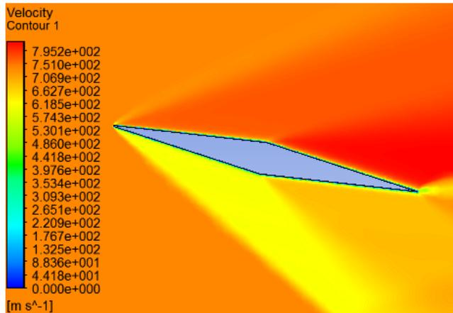
Figure 16. Distribution of airflow velocity around the airfoil at the angle of attack  $12^\circ$
