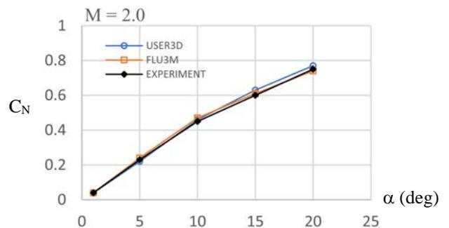
Figure 14. Variation of normal force coefficient for one fin with angle of attack [6]
