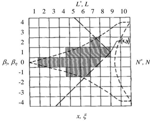
Figure 7. Wing coordinate system [3]
