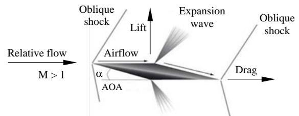
Figure 6. Airflow around a supersonic fin
