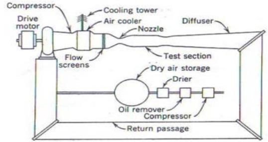
Figure 10. Continuous Wind Tunnel [8]
