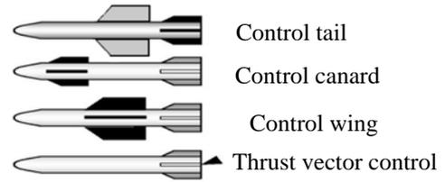
Figure 1. Four main categories of missile controls [1]
