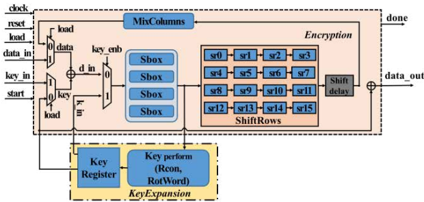
Figure 1. AES 32-bit datapath architecture using 4-Sbox for both Encryption and KeyExpansion procedure.
