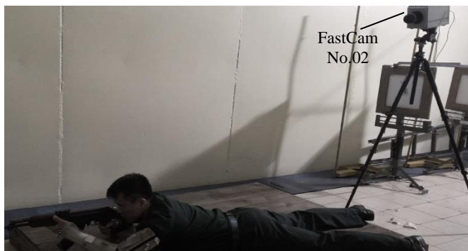
Figure 10. Location of camera for barrel horizontal displacement record
