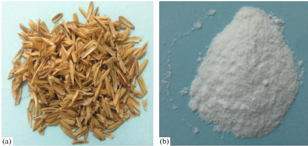
Fig. 1. (Color online) Pictures of (a) rice husk and (b) extracted nano-silica.
