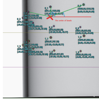
Fig. 4. Method to label balls in projection image. For each group, the virtual center is first calculated, then the angle of each ball with the horizontal axis crossing virtual center will be calculated and used to determine its label. The cross sign indicates the centroid calculated using ellipse fitting technique.
