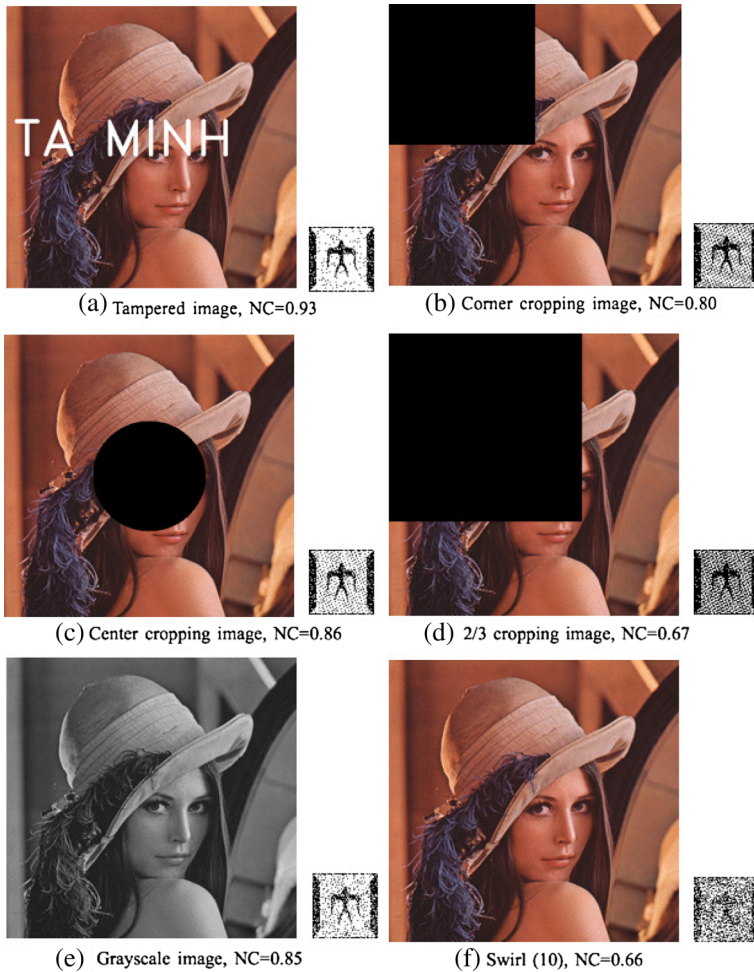
Fig. 16 Some examples of simulation results against common image processing attacks on Lena image ( \{q = 1.2, Q = 0.40\} )
