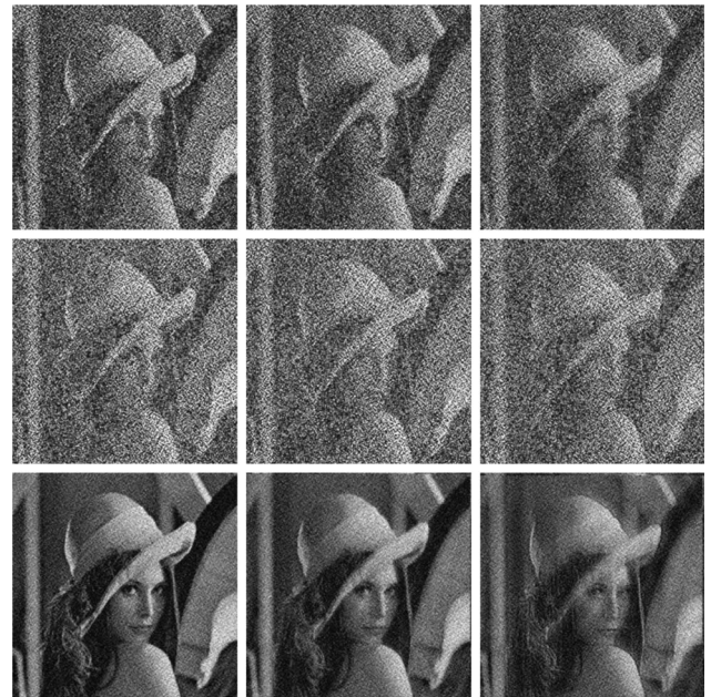
Fig. 7. Simulated decoded images when the SNR is 10 dB and the ratio factor \gamma is 0.9. Top to bottom: PM1, PM2, and the subtraction method. Left to right: \psi = 0 , \psi = 15 , and \psi = 30 .
