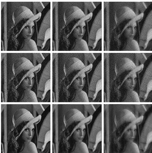
Fig. 6. Simulated decoded images when the SNR is 20 dB and the ratio factor \gamma is 0.8. Top to bottom: PM1, PM2, and the subtraction method. Left to right: \psi = 0 , \psi = 15 , and \psi = 30 .
