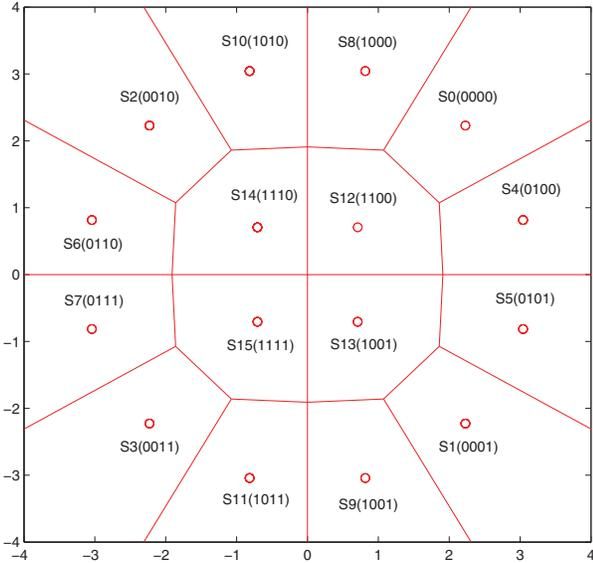
**Figure 3: The conventional 16-APSK as defined in the DVB-S2 standard.**
