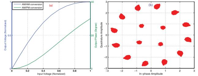
Figure 2: a). AM/AM and AM/PM conversion characteristics; b). The 16-APSK conformed to the DVB-S2 standard after being passed through the HPA.
