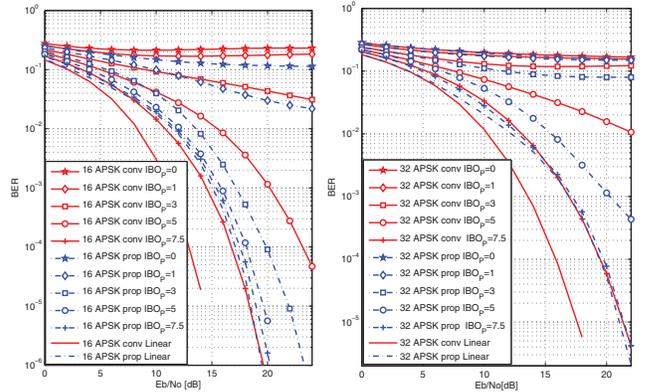
Figure 7: Simulated BER performance of the proposed APSK and the conventional APSK in linear and nonlinear conditions.
