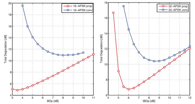
Figure 9: Total degradation ( $TD$ ) versus peak input backoff power ( $IBO_P$ ) at  $BER = 10^{-3}$  of the proposed system and the conventional one.
