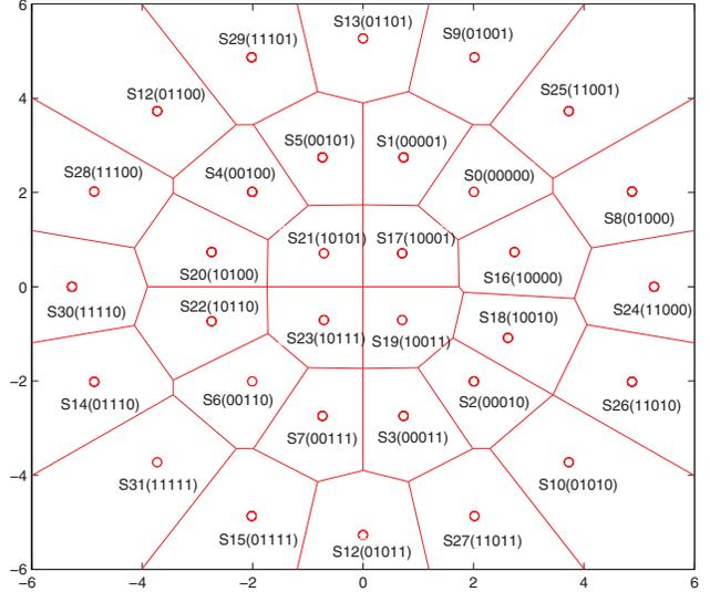
**Figure 4: The conventional 32-APSK as defined in the DVB-S2 standard.**
