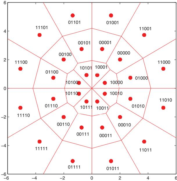
Figure 6: The proposed signal constellation and its mapping for the 32-APSK.
