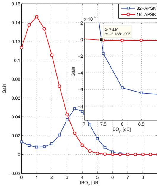
Figure 8: The BER gain of the proposed APSK compared to the conventional APSK at  $Eb/N_0 = 20$  [dB].
