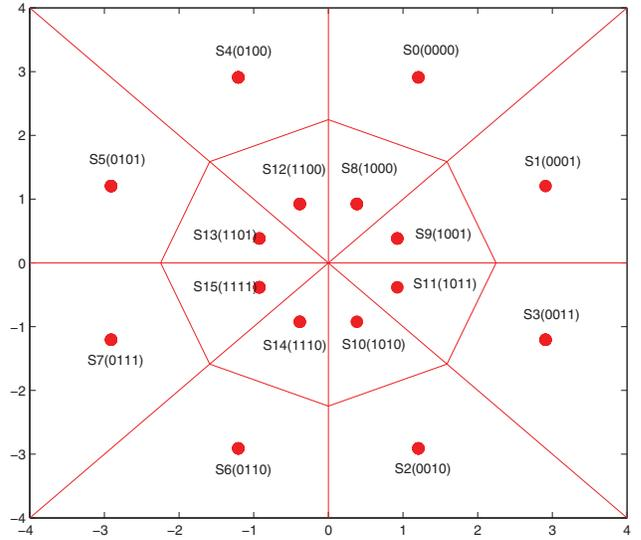
**Figure 5: The proposed signal constellation and its mapping for 16-APSK.**
