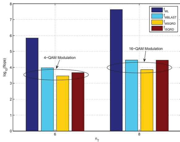
Fig. 2. Complexities of ML, MBLAST, MSQRD, and ISQRD detectors in different MIMO configurations; 4-QAM and 16-QAM modulation.
