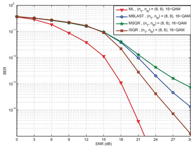
Fig. 4. BERs of a HR-SM scheme with  $n_T = n_R = 8$  when using the ML, MBLAST, MSQRD, and ISQRD detectors; 16-QAM modulation.
