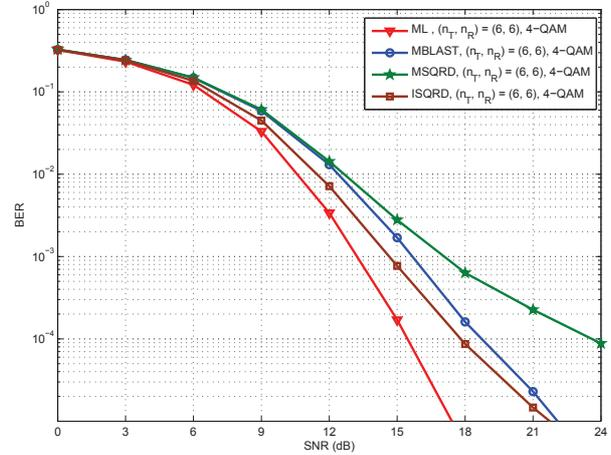
Fig. 3. BERs of a HR-SM scheme with  $n_T = n_R = 6$  when using the ML, MBLAST, MSQRD, and ISQRD detectors; 4-QAM modulation.
