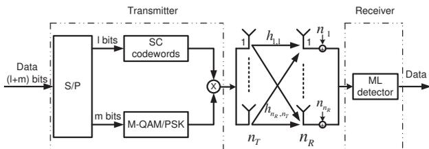
Fig. 1. Block diagram of a HR-SM system
