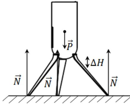
Figure 4: Forces impacting on damper shafts during connecting to ground
